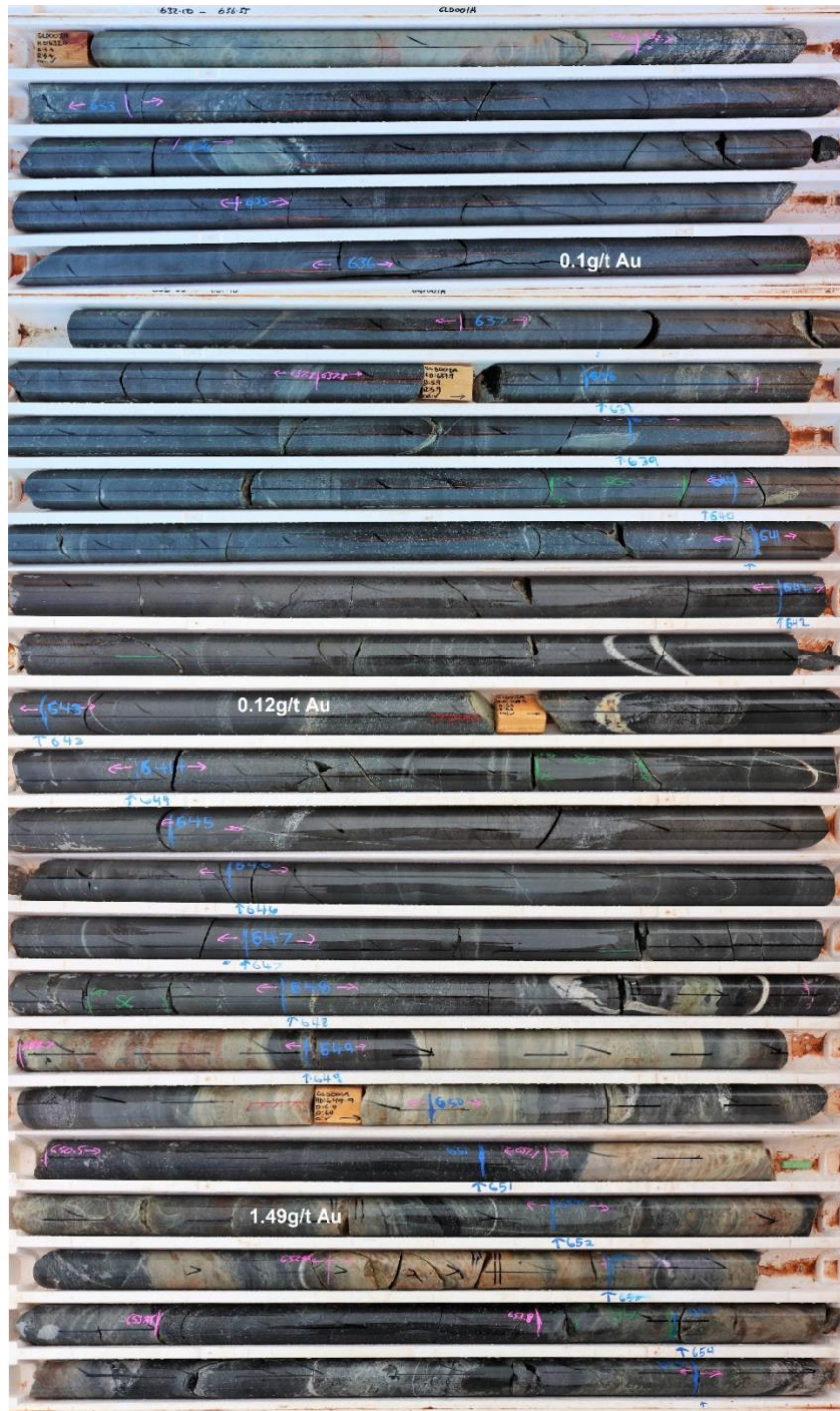
Figure 4. GLD001A Drill core highlighting pale, calcareous alteration, metasediments and the darker, magnetic mafic – intermediate igneous intrusive rocks; with anomalous assays written in white
