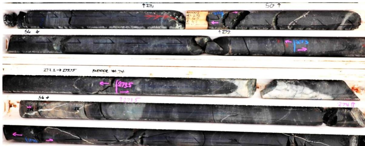
Figure 2– BHD002 - High grade Quartz vein structure; 0.6m @ 2.56g/t Au from 273.5m.
