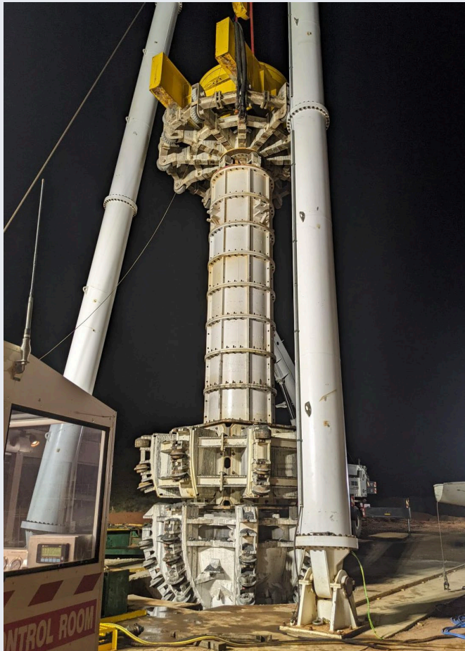
Newcrest bringing its word class expertise to the Havieron project with a blind-bore shaft (above image).
